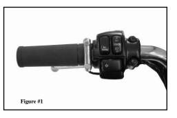
Route the wires from the dual button handlebar control bracket neatly along handlebar into the speedometer/tachometer area or inside the handlebar into the speedometer/tachometer area. From there run the wire assembly under the frame towards the battery. Alongside the battery is the approximate location that the control module will be mounted. Make sure to secure the wires along their routing with wire ties provided. Excess wire can be coiled and hidden in the battery area.
